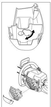
IMPORTANT! If the temperature rises above -5°C (23°F) or 0°C (32°F) respectively the saw MUST be restored to its normal settings. Otherwise there is a risk of overheating, which can cause severe engine damage.
